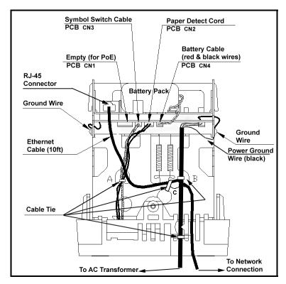
Figure 2-8. Rear View Showing Cable/Connector Location.
